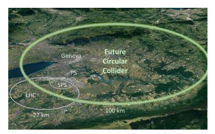
The FCC would have a circumference of 100 kilometers four times that of the existing LHC and have 10 times the atom-smashing power. CERN released its conceptual design and report in January 2019. Researchers hope to
